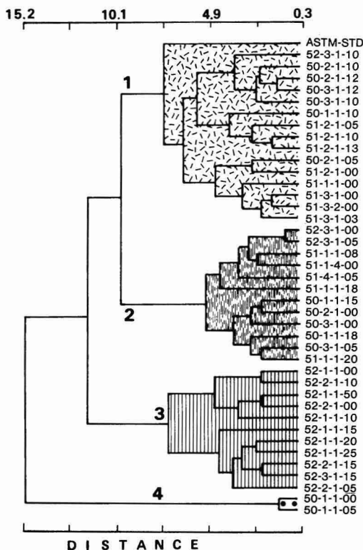
FIGURE 11a. Classification of north shore Oahu sand samples and ASTM standard distribution for sand for aggregate.
