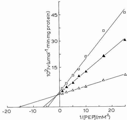
FIGURE 1. Double reciprocal plot showing the pattern of inhibition by ATP with respect to phosphoenolpyruvate (PEP) for pyruvate kinase from the spadix. LEGEND:  $\Delta$ , 0 mM MgATP;  $\blacktriangle$ , 2.5 mM MgATP;  $\square$ , 5.0 mM MgATP. OTHER CONDITIONS: 2 mM ADP, 10 mM  $MgSO_4$ , 100 mM KCl, 100 mM imidazole HCl, pH 7.0, 25°C.
