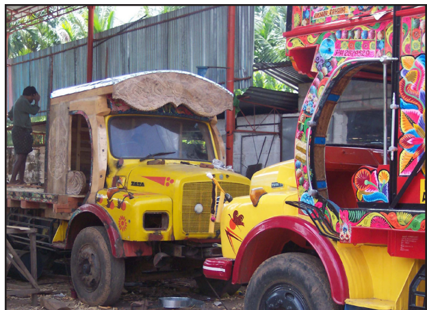
Figure 20. Body building of trucks by wild jack timber in a local work shop.
