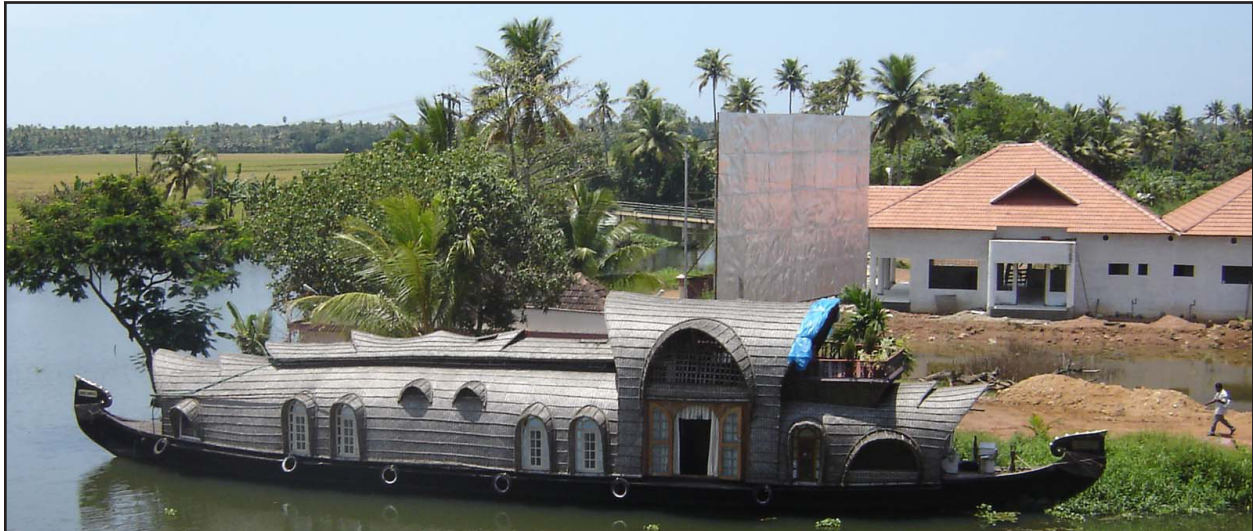
Figure 32. An old cargo boat of wild jack wood converted into a luxury house boat as viewed from Alappuzha.
