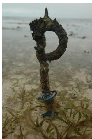
Autonomous iBTag™ submersible temperature loggers attached to permanent site marker at Green Island (GI1)
