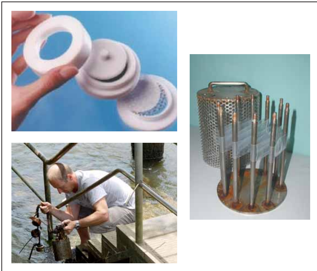
Figure 10. Passive samplers used to collect time integrated pesticide samples from rivers and ocean sampling sites (ENTOX, D. Haynes).
