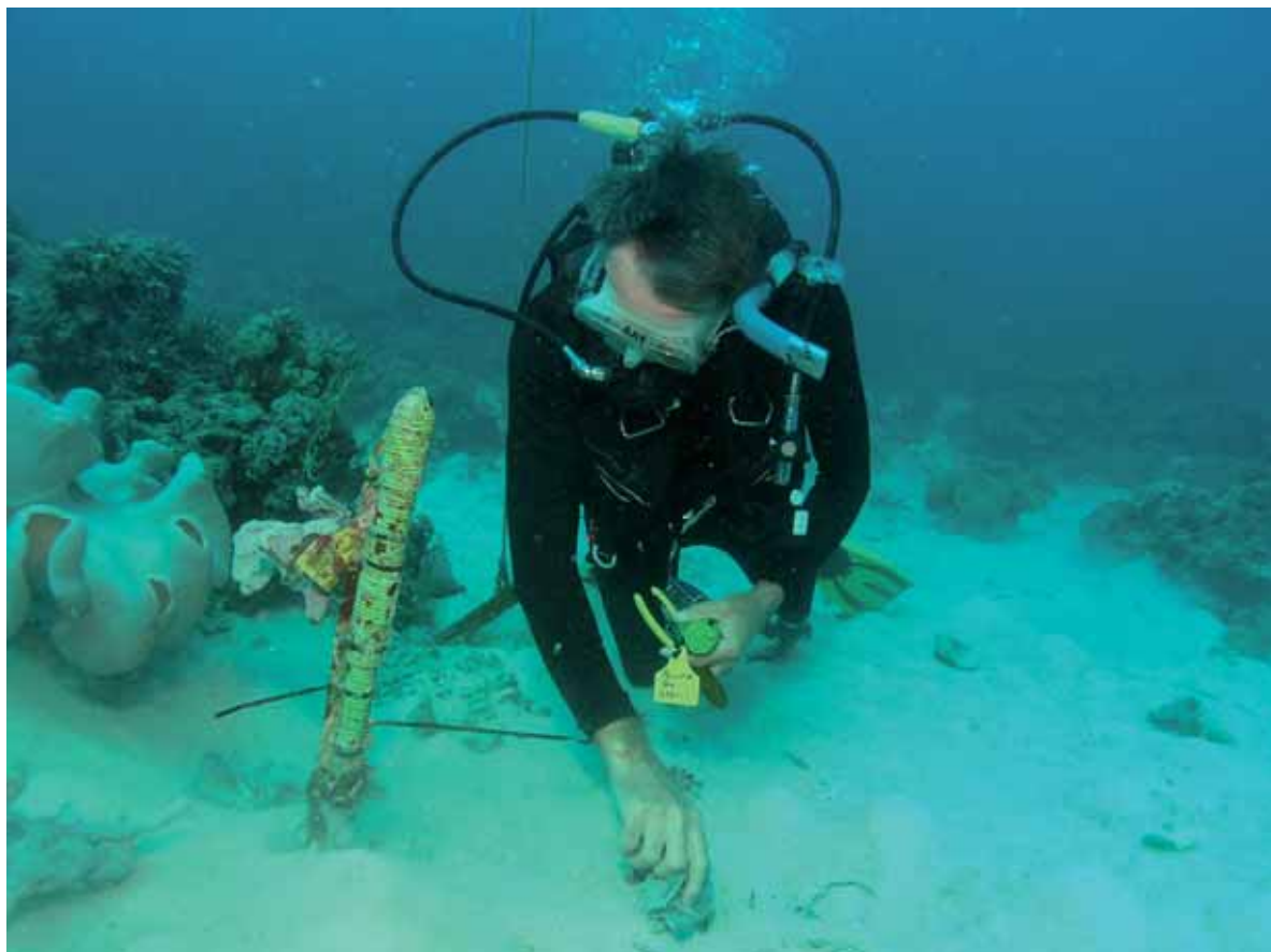
Figure 16. In situ seawater temperature logger (AIMS).
