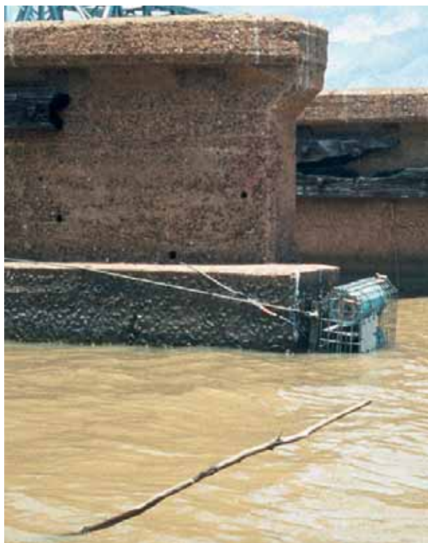
Figure 9. River turbidity logger (M. Furnas).
