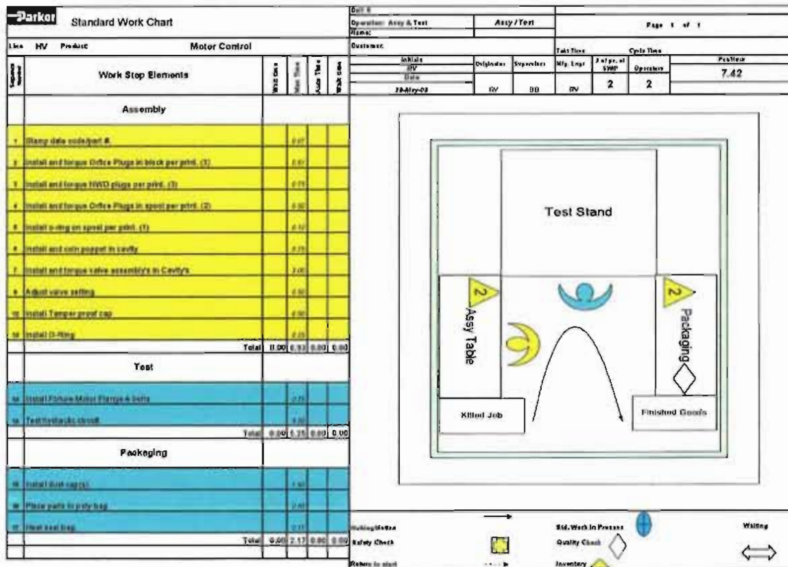
Figure 6. Example of Standard Work for an Assembly Cell
