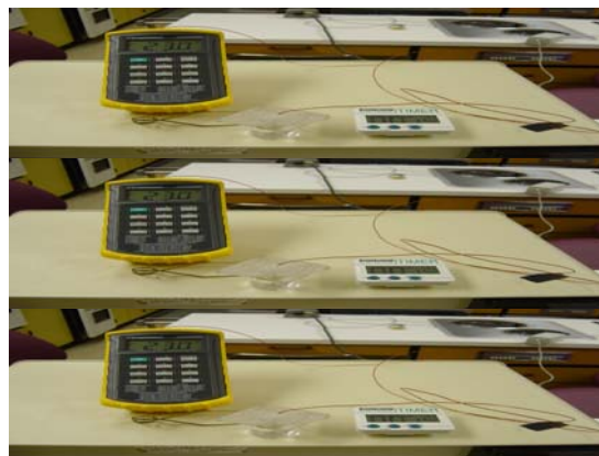
Figure 3 – Thermocouple set-up attached to digital thermometer
