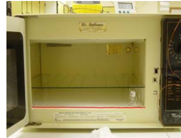
Note: Glass height signified by red line Level 1 = 0 inches off the bottom
