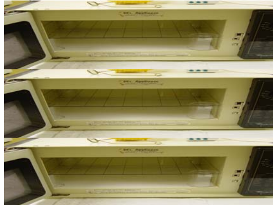
Figure 15 - Glass grid elevated to the third level
