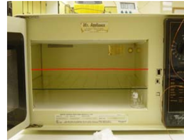
Note: Glass height signified by red line Level 3 = 3.00 inches off the bottom
