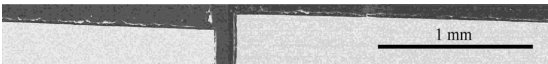
Figure 5-4 B : Transversal cut of the T91 steel after fatigue failure in liquid Pb-Bi at 300°C, \Delta\varepsilon_t = 2.2\%
