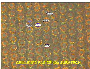
Figure 2. A microscope photo of a copper micromesh produced by laser machining: holes are 14 \mu\text{m} diameter with a pitch of 40 \mu\text{m} . The concept of a PIM photon detector with a reflective photocathode.
