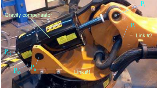
Fig. 1. Gravity compensator of robot KUKA KR-270 TM
