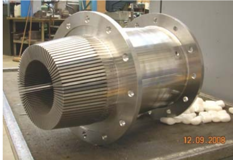
Figure 10.4.4. Drag enhancer device for the windowless spallation target.
