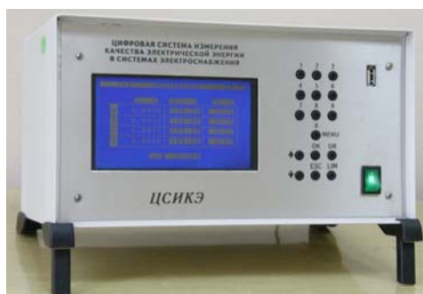
Fig. 1. Digital system for the measurement of electrical energy quality (DSMEEQ)
