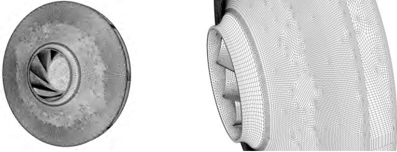
Figure 7 – The computational mesh of the impeller surface of the blower aggregate BA_I
