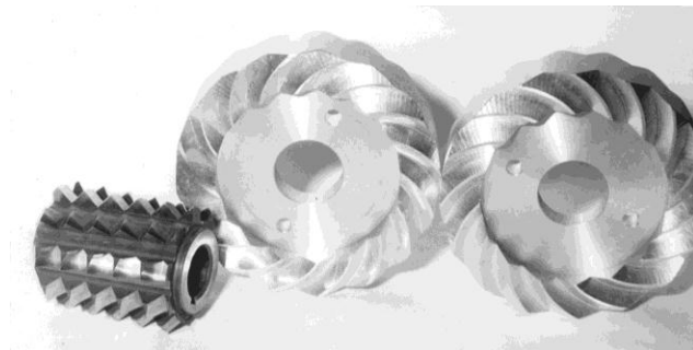
Fig. 5 – Experimental involute spiral face coupling mating flanges and hob (the same hob was used to machine both right and left hand spiral face gears)
