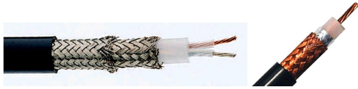
Fig. 9. Double shielded cable. Left – with double braided screen; right – with double combined shield (braided screen and foil)
