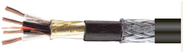
Fig. 11. Cable RE-2X(ST)2Y(Z)Y PIMF characterized as interference superstable (transmitting analogue and digital signals up to 200 kbit/sec; pair-twisted wires, each pair shielded with PE foil; three-layer common foil shield armored with steel wire; external XLPE isolation; up to 24 pairs of wires per cable; can be used outdoors and for burial; has high mechanical strength)
