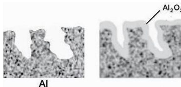
Fig. 2. Surface of anode foil after electro-etching
