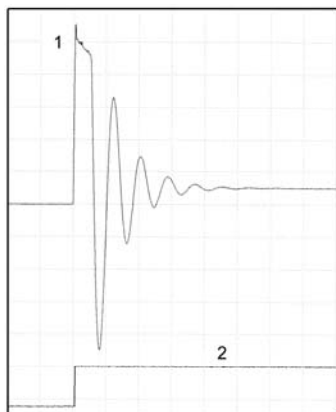
Fig. 6. Oscillogram of input/output signals in device during laboratory testing with a low-voltage simulator of high currents. 1 - the pulse of a current generated by a simulator; 2 - a signal on device output
