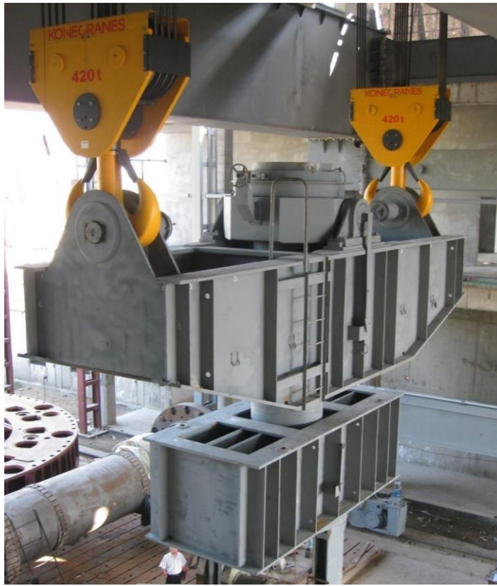
Fig. 7. Cross/radial/transverse cross arm/bar for the concerted operation of the main hoist mechanisms
