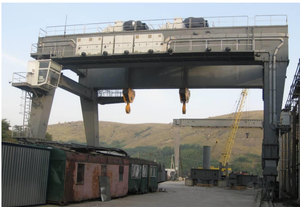
Fig 5. portal bridge special-purpose crane with the load-carrying capacity of 420/420/16 t. Technical properties: operating mode group as to ISO 4301/1 is A2; the main hoist load-carrying capacity is 840 t, the accessory hoist load-carrying capacity is 16 t; the main hoist height is 56 m, that of the accessory hoist is 76 m; the crane span is 20,5 m; the crane foundation is 12,75 m; mechanisms velocities: that of the main hoist is 2,4 m per minute, that of the accessory hoist is 12,6 m per minute, that of bogey travel is 10,02 m per minute, that of bogey travel for accessory lifting is 4,98 m per minute, that of crane travel is 19,8 m per minute; main hoist mechanism velocity regulation scope is 1:100, that of the rest of the mechanisms is 1:50; crane mass is 450 t.
