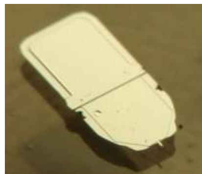
10. Ábra. Olympus AC160TS-C2 microcantilever.
