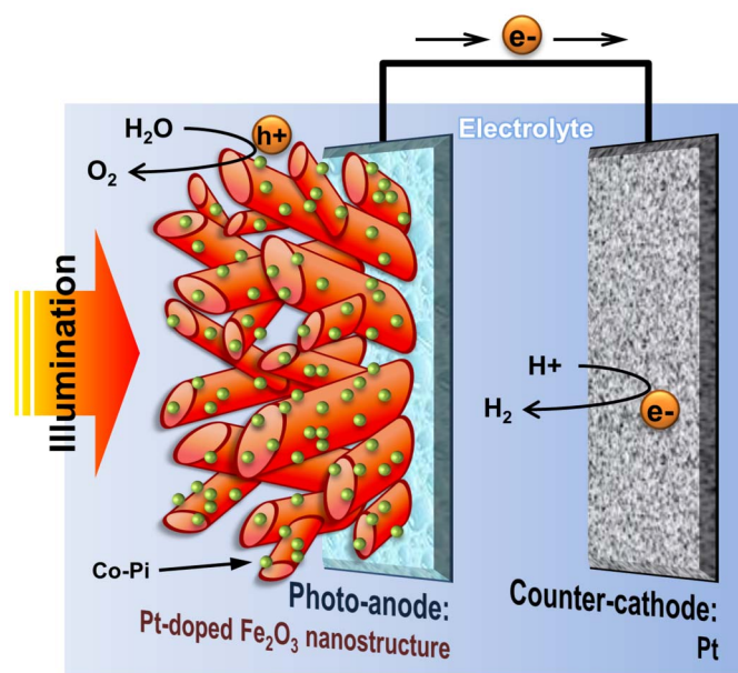
Figure 1 | Schematic diagram for a photoelectrochemical cell with the hematite thin film photoanode. The anode has Pt-doped, highly crystalline worm-like nanostructure modified with Co-Pi as an oxygen evolution co-catalyst on its surface. Charge recombination can be effectively suppressed with the help of the promoted charge separation at both the inside and outside of the photoanode by Pt-doped nanostructure and Co-Pi loading, respectively.
