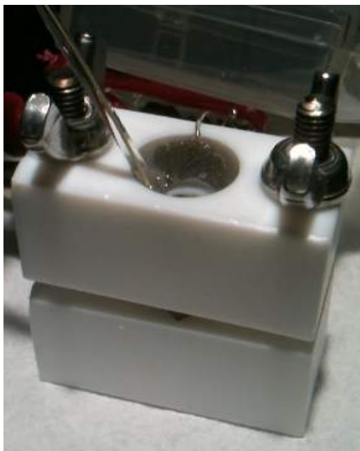
Figure S6. Experimental setup for PEC measurements
