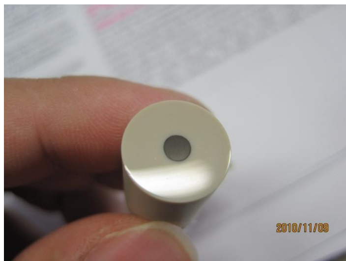
Appendix Figure 2-3. As-prepared catalysts thin-film.
