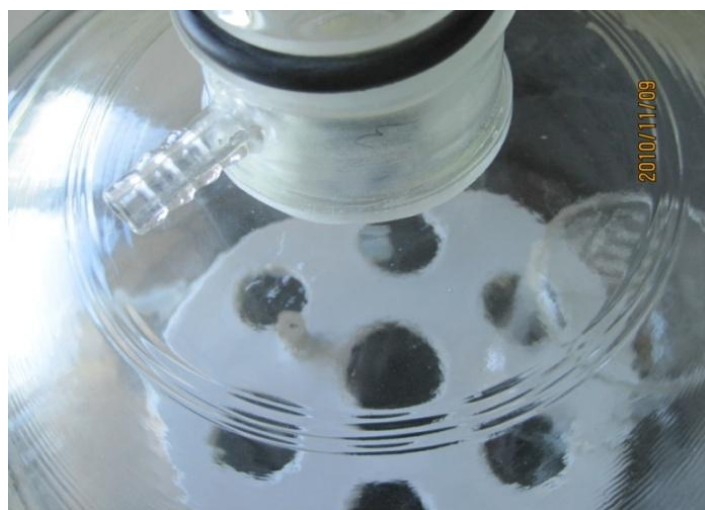
Appendix Figure 2-2. Vacuum drying for the preparation of catalysts films.
