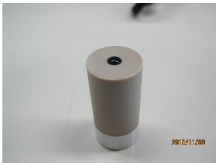
Appendix Figure 2-1. Loaded aqueous catalyst ink onto glassy carbon electrode.
