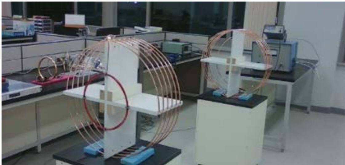
Figure 1-3: Magnetic resonance wireless power transfer.
