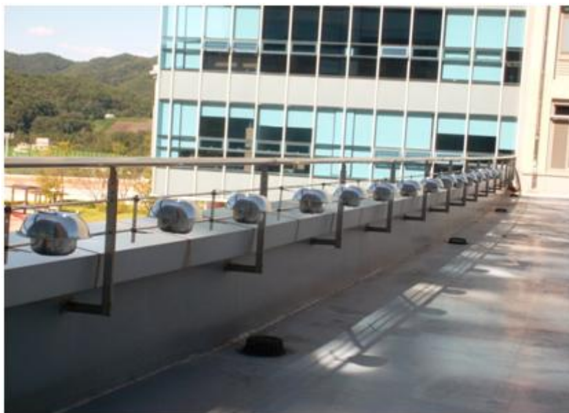
Figure 12. Passive air sampler for collecting particulate and gaseous phase PAHs
