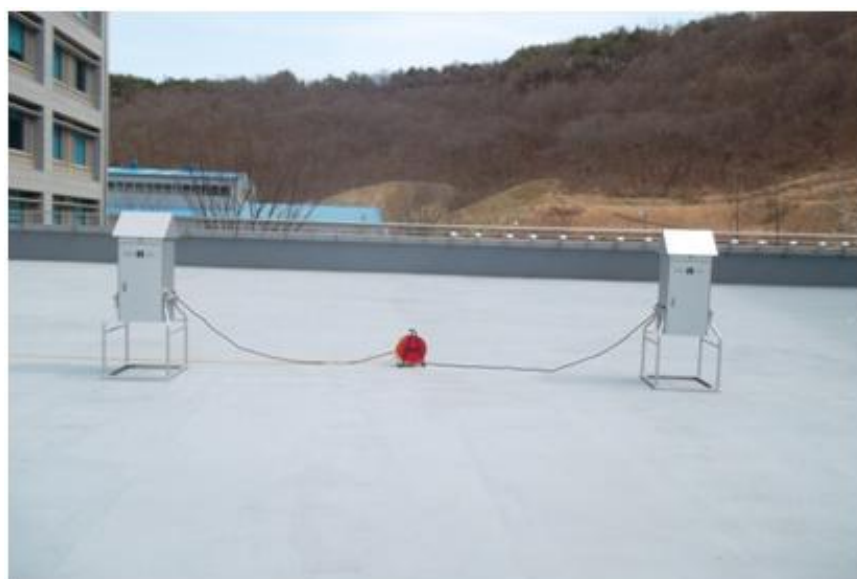
Figure 11. High volume air sampler for collecting particulate and gaseous phase PAHs
