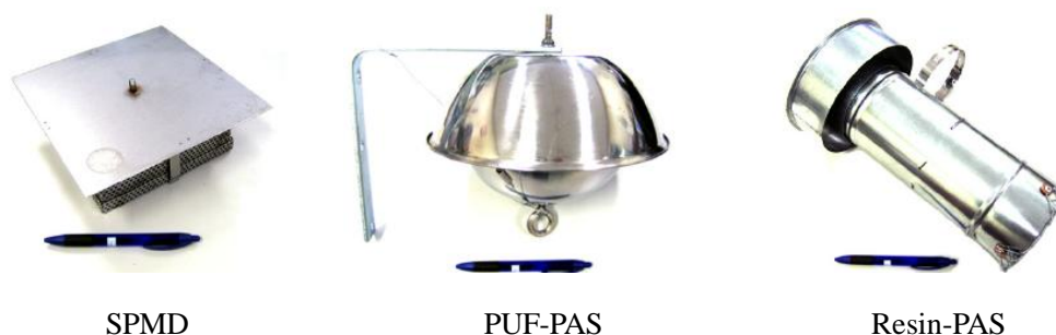
Figure 6. Representative passive air sampler which developed in previous studies
