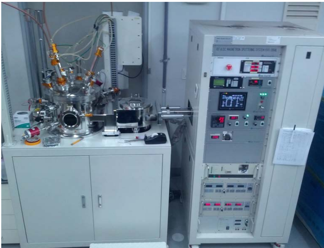
Figure 2.1 Radio Frequency Sputter (RF-sputter).
