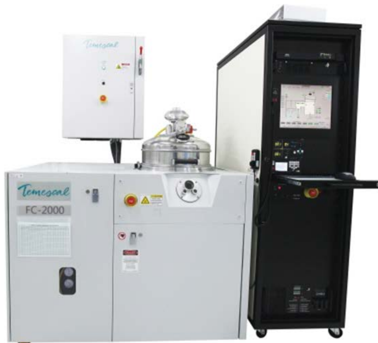
Figure 3.1 E-beam evaporator, Pd nanoparticle and electrode, Au/Ti (200/20nm) deposition.
