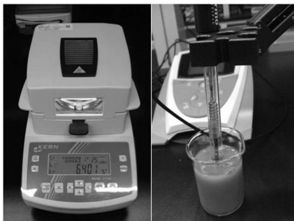
Figure 8: The measurement process of pH and moisture content
