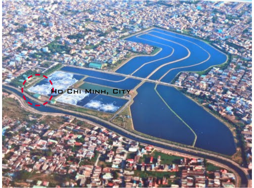
○ Located within one of the denser urban environments in the world, the Aerated Lagoon Park purifies runoff and wastewater from the surrounding watersheds.
