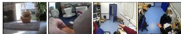
Fig 2. Various camera configurations and their associated field of view. (a) Chest-mounted. (b) Camera at manipulation level. (c) Shoulder-mounted. (d) Head-mounted, viewing down.
