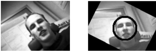
Fig. 8. Face detection after geometrical correction. On the original frame (left) the face detector fails to detect the face, while on the rotated image (right) it detects the face.
