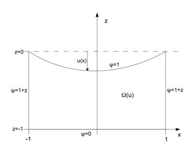
FIGURE 1. Idealized electrostatic MEMS device.
