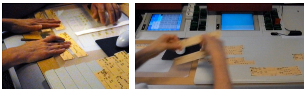
Figure 7: a) one stack in each hand; b) bi-stack bi-manual strip transfer from the planner board to the tactical one.
