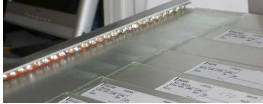
Fig. 5. Infrared lights along one side of the strip board
