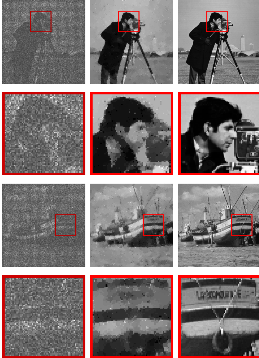
FIGURE 10. Reconstruction of the images “cameraman” (first and second rows) and “boat” (third and fourth rows) with a noise level \sigma = 0.2 . The remaining parameters are set as follows: \bar{w} = 16.2 , \sigma_c = 0.81 and \sigma_w = 0.07 . The left column correspond to partial available data where each pixel is assigned its maximum intensity over all k \in \{1, \dots, K\} . The middle and right columns correspond resp. to the image estimate and the ideal image. Detailed views of all these images are also provided on the second and fourth rows.
