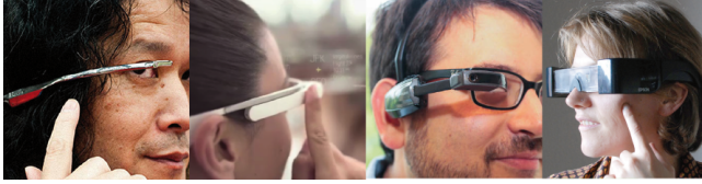
Figure 2. HWDs ordered by increasing temple size: Telepathy [30], Google Glass [6], Vuzix M100 [31] and Moverio [4].
