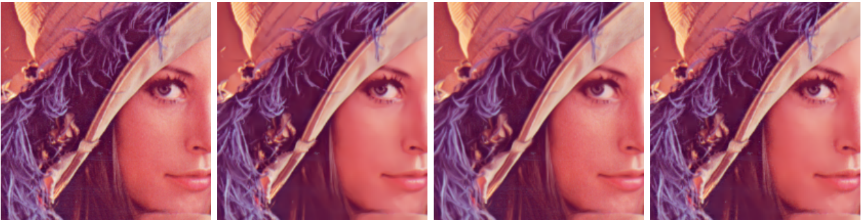
Figure 6: I: Detail of the Lena image. II: cEED removes noise and preserves most image detail. III: cCED enhances the flow structure of the hat plumes, without much affecting the rest of the image. In particular it does not remove noise. IV: Isotropic diffusion (10, Perona Malik like) removes noise in the interior of the image regions, but leaves some noise close to image contours such as the border of Lena's cheek. Parameters: T = 2 , \lambda = 0.003 , m = 4 , others default.
