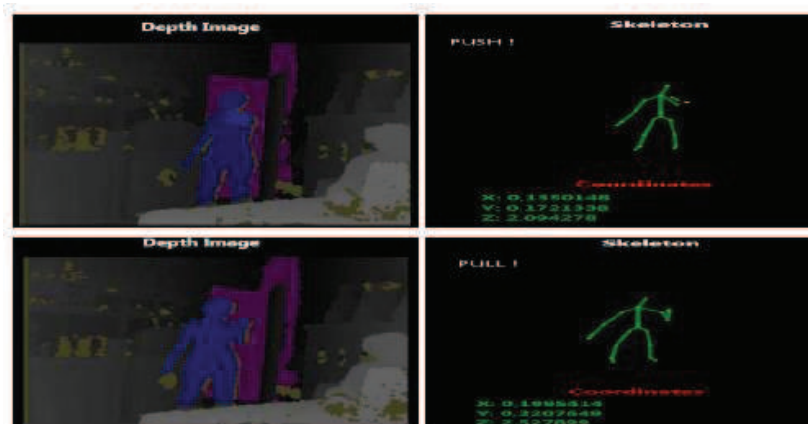
Figure 4: Recognition of push and pull gesture
