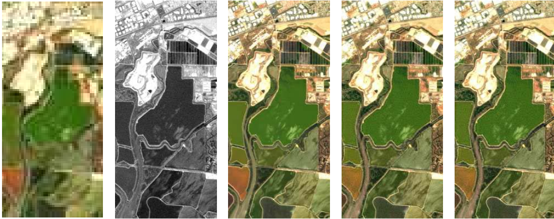
Fig. 4. Hyperspectral pansharpening results. 1st column: HS image. 2nd column: PAN image. 3rd column: Reference image. 4th column: ADMM [23]. 5th column: Proposed method.
