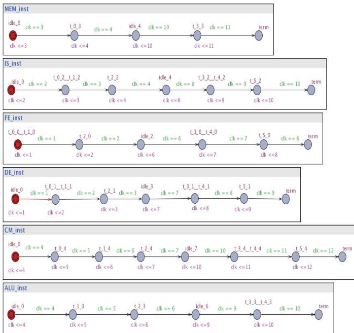
Figure 3: Stage view network timed automata
