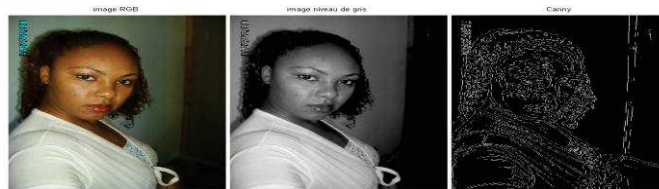
Fig. 9..Edge detection using Canny filter on grayscale image
