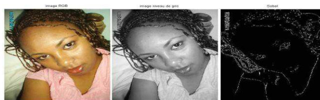
Fig. 8.. Example of edge detection using the Sobel filter
