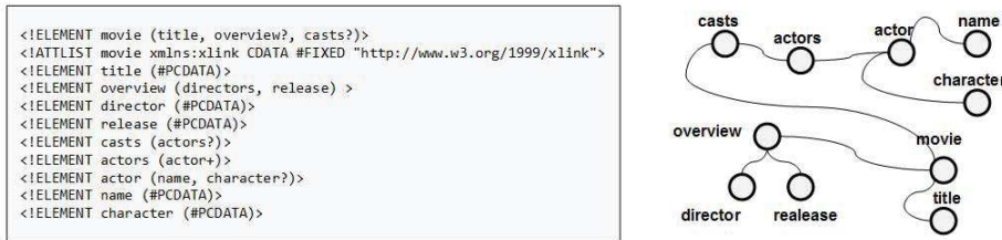
Fig. 3. Example of a “movie” DTD with its corresponding graph
