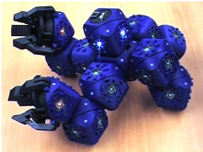
Figure 2: A chain type modular robot composed of molecule-like modules and grippers.
