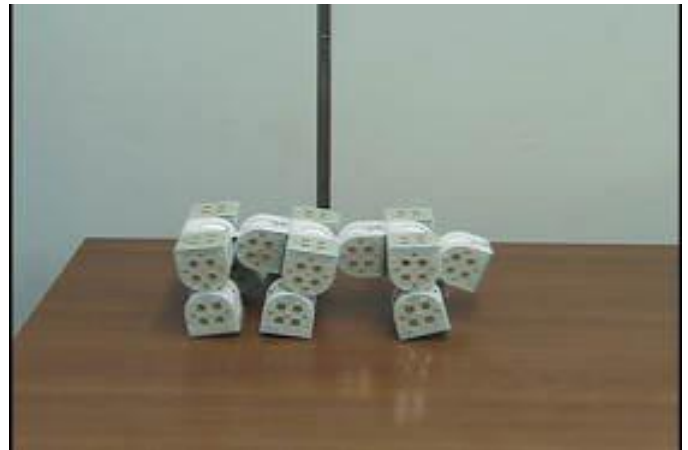
Figure 3: A six legs hybrid M-TRAN 9 modules robot.
