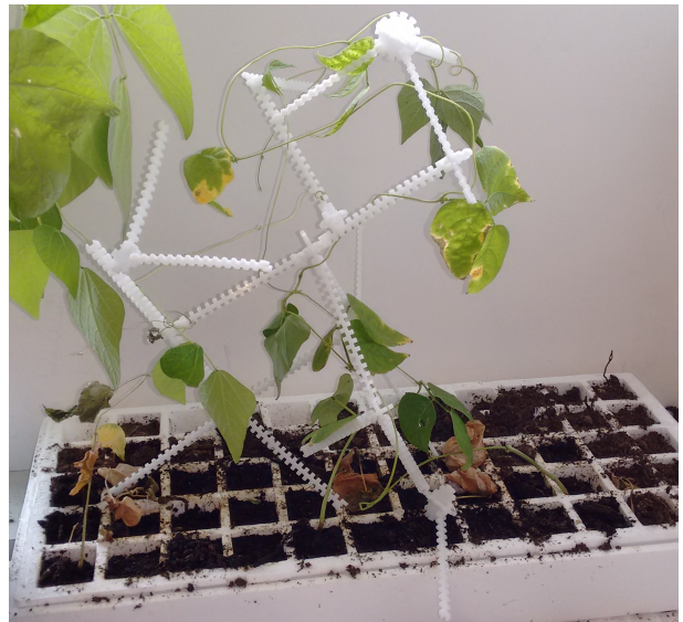
Fig. 5. Prototype of the flora robotica rods and nodes without the electronics.
