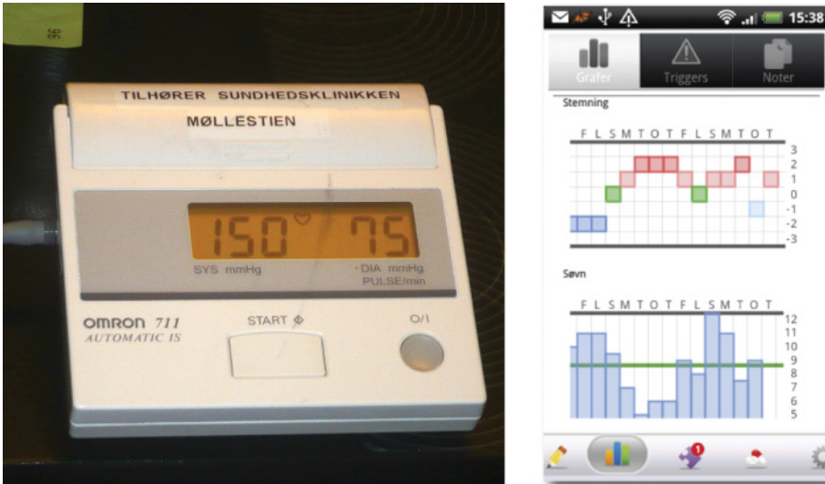
Fig. 3. Two interfaces providing health information are displayed. On the left, a blood pressure monitor displaying blood pressure values. On the right, an overview of mood and sleep levels over a period of time from MONARCA [Bardram et al. 2013], ©ACM.
