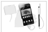
**Figure 1:** Cradle with a built-in camera and light sources designed to fit a modern smartphone.
