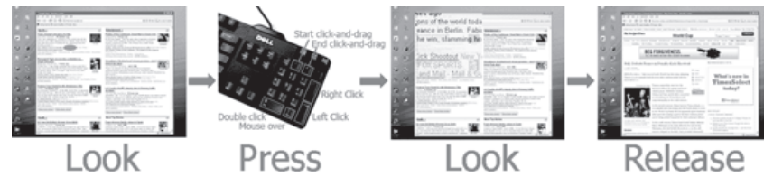
Figure 5.3: The EyePoint selection method [85] uses a two-step process, first fixating on a target and then pressing a keyboard shortcut. This will bring up a zoomed-in view around the last fixation, which allows higher tolerance for eye tracker noise. The user fixates on the target again and releases the button, which issues a simulated mouse click in the position of the current fixation.
