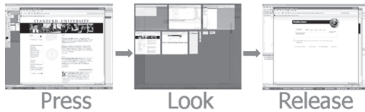
Figure 5.4: The EyeExposé window selection method [83] supports fast application switching. The interaction combines the use of keyboard input and gaze pointing.
