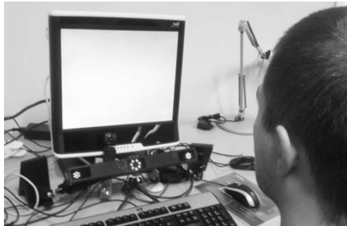
Figure 4.4: Experimental setup. The participant is conducting the test using the Mirametrix system. Throughout the experiments the monitor from the Tobii T60 system was used for consistency.
