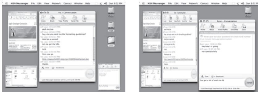
Figure 5.5: EyeWindow by Fono and Vertegaal [36]. On the left, gazing at the bottom right window makes it bigger and moves the focus to that window, so that (on the right) typing can continue without removal of the hands from the keyboard.
