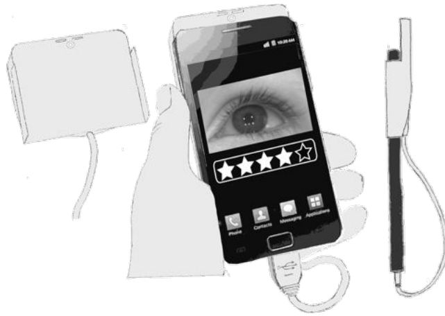
Figure 9.4: Cradle with a built-in camera and light sources designed to fit a modern smartphone.
