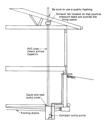
Figure 7. Soil depressurization by suction on sump hole.
