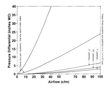
Figure 10. Pressure vs airflow curves for different aggregates.
