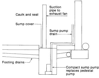
Figure 8. Converting a sump hole into a radon collection sump. Be sure to caulk all joints between materials.
