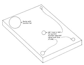
Figure 9. Place test opening at strategic locations around slab to insure that a suction exists at all locations. Be sure to caulk holes after completing the test.
