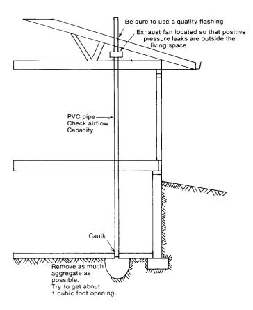
Figure 6. Depressurization of the soil by applying suction to the aggregate below the slab.
