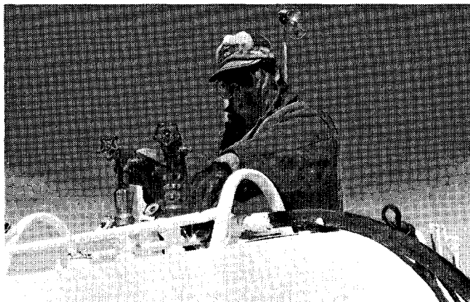
Goggles and long gauntlet rubber gloves are worn for all ammonia equipment contact operations.
