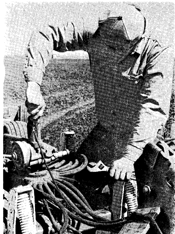
Never attempt field repairs on ammonia metering equipment. This chore is reserved for clean work benches and trained repairmen.
