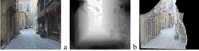
Fig. 3. An example of a depth map (b) extracted from the Street video sequence, the associated vrml model (c) and the corresponding image in the sequence (a).
