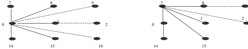
(b) Neighbors and interfering nodes shown with lines and dashed lines respectively for node 0 and 7
