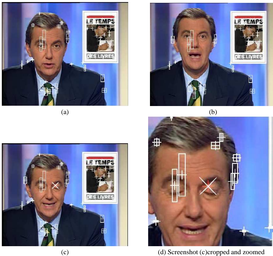
Figure 1: An example of categories of points of interest according to their behaviour: the boxes represent the amplitude of moving points along the trajectory (motionless points do not have box). The "+" correspond to the mean position of such points. The "x" shows a spatio-temporal rare point (the eye blinking).
