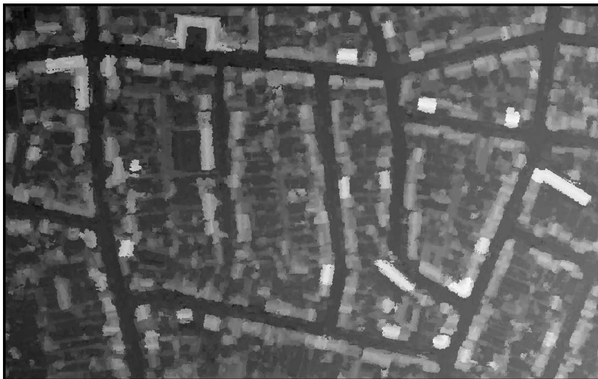
Figure 23: Digital Elevation Model of a part of Rennes, France (©IGN). This DEM has been constructed by aerial stereovision.
